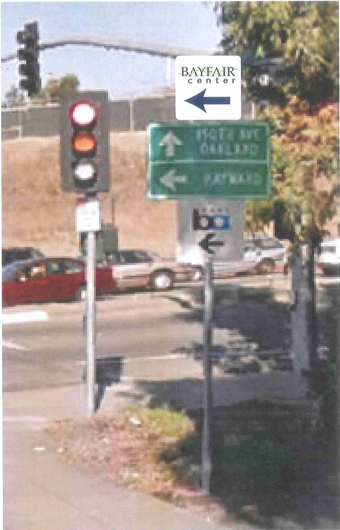
Bayfair Directional Foothill Blvd. and Fairmont 24"x24" .063 aluminum w/rounded corners. Graphics printed on 3M ij680CR Reflective Vinyl Laminated with Oraguard 290G 8yr+4UV Gloss Laminate
