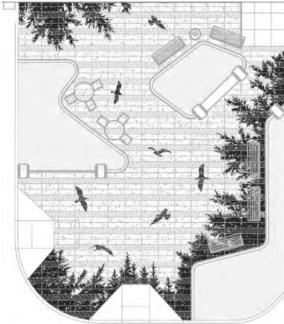
Overhead view of sandblasted design in concrete for the plaza area.
