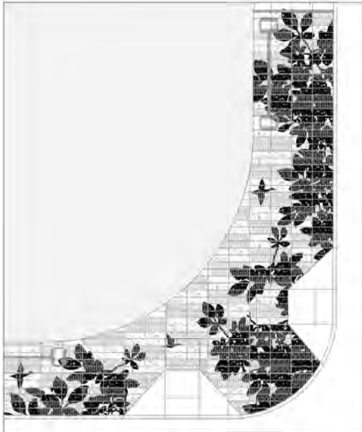
Overhead view of sandblasted design in concrete for the Sidewalk area.
