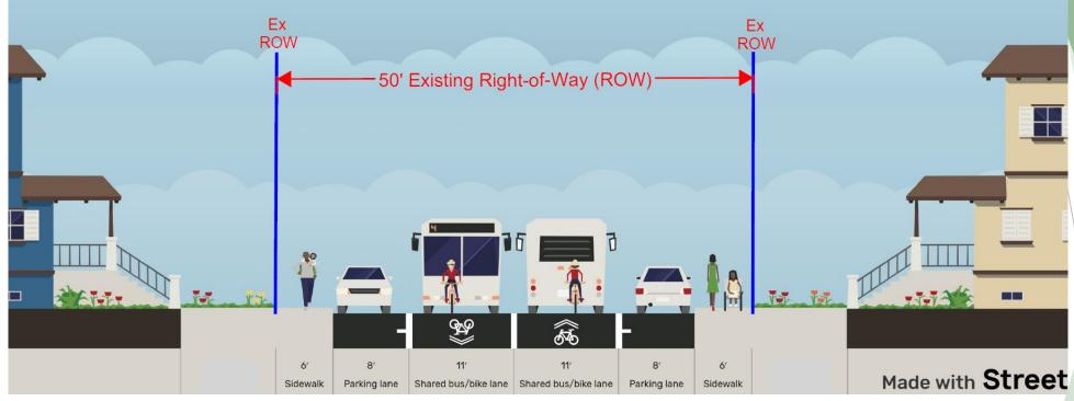
This typical section shows the project features for Alternative #1. The dimensions shown are preliminary and may change to accommodate local site conditions.
