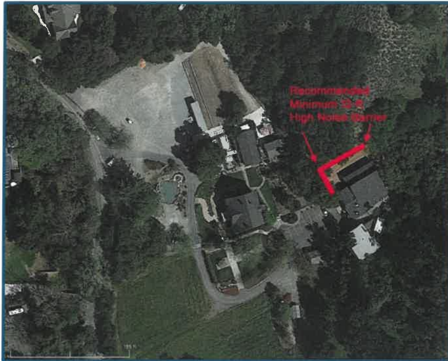
Figure 8. Recommended 12-ft High Noise Barrier at Event Center
