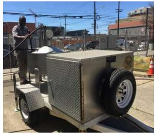
A Weights and Measures inspector uses a 100 gallon gas prover to test high-flow fuel meters used at airports or truck stops. These programs protect consumers and preserves equity in the marketplace by directly testing commercial devices used in consumer transactions.
