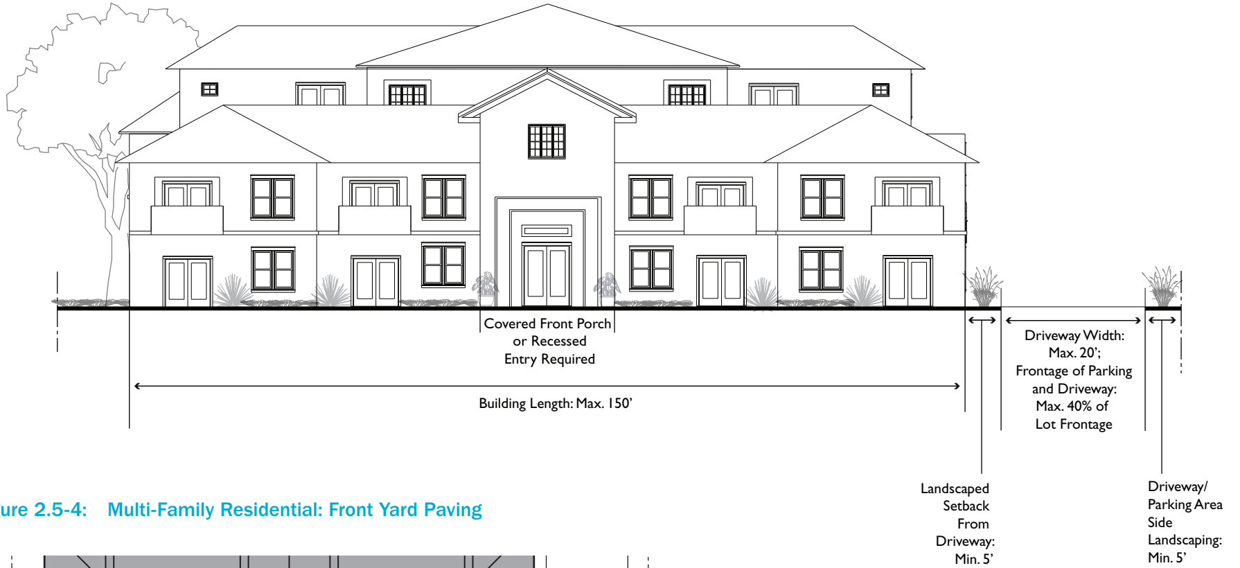
Figure 2.5-3: Multi-Family Residential: Elevation
