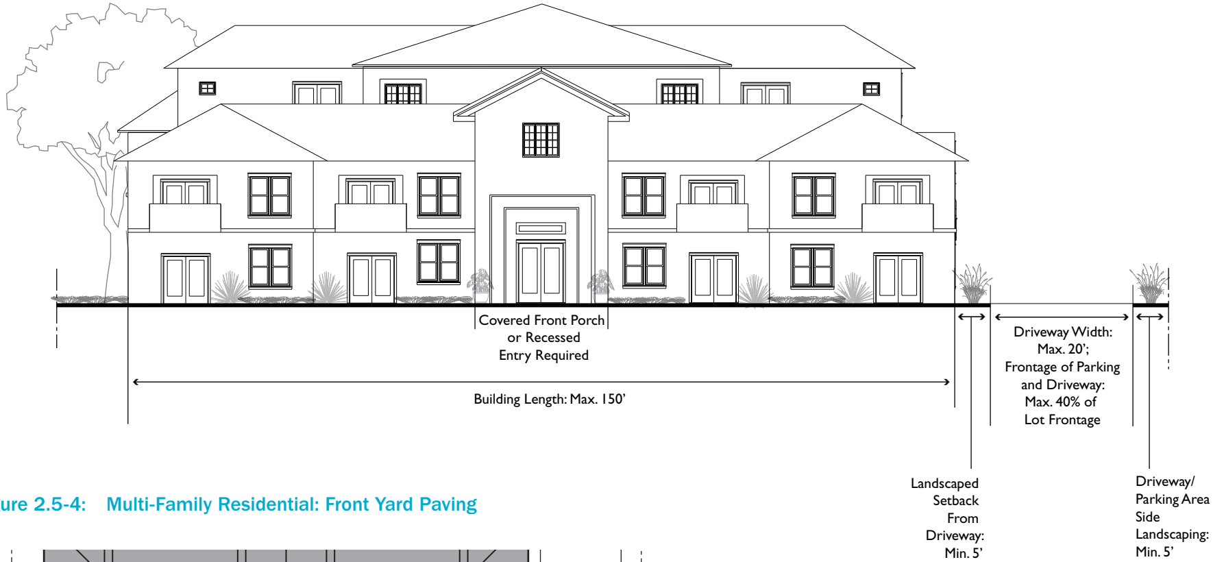
Figure 2.5-3: Multi-Family Residential: Elevation
