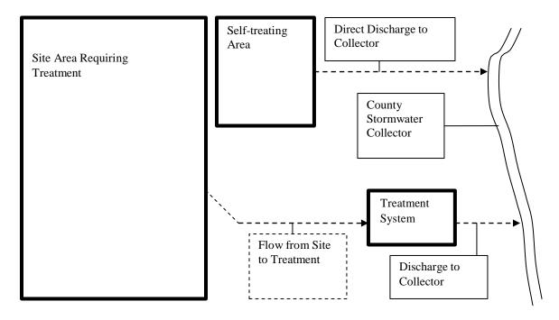
• "Alternative surfaces," if properly designed, can reduce the amount of flow from the site to the treatment measures by enabling infiltration of some of the stormwater to the underlying soil; however, the use of such designs must be recommended by the project geotechnical engineer in the preliminary
