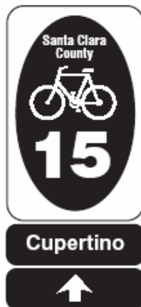
Route sign with destination Caltrans SG-45 with supplementary placards
