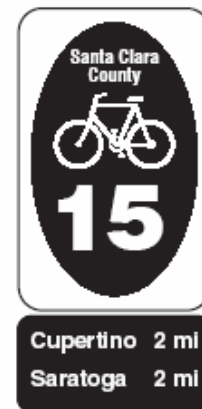
Route sign with distance Caltrans SG-45 with supplementary placard
