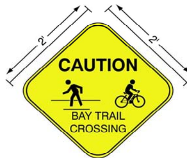
SW 1 Trail Crossing Warning Sign (Black on Yellow)
