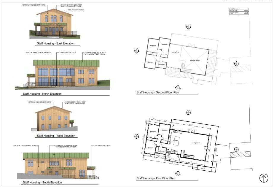
Figure 3-11 Staff Housing - Floor Plans and Elevations
