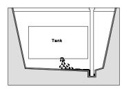
When installed and operated according to the manufacturer's specifications, secondary containment with interstitial monitoring meets the federal leak detection requirements for USTs. Operation of the monitoring device at least once each month fulfills the requirements for the life of the tank. Secondary containment with interstitial monitoring can also be used to detect leaks from piping (see the section on leak detection for piping starting on page 22).
