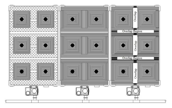
Figure 31 – Typical Flow Balancing Problem (See Below)
