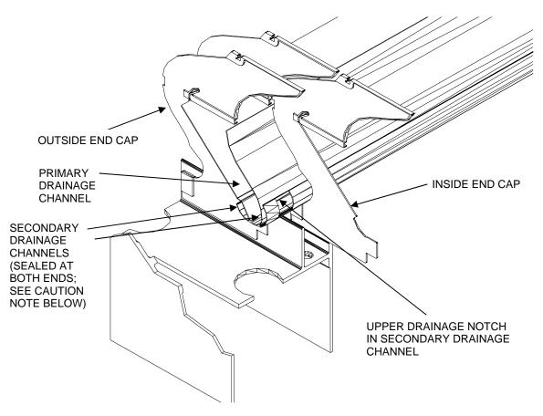
Figure 42 – Close-Up View: Water Collection System
