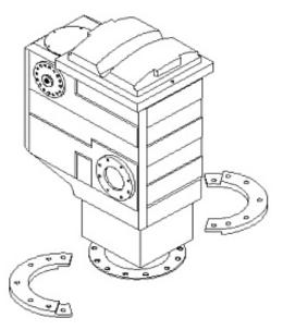
Figure 25 – Discharge Flange and Split Ring
