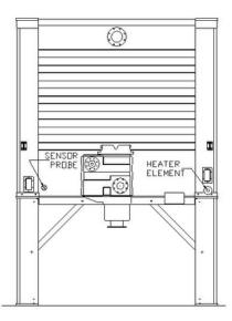
Figure 15 – Immersion Basin Heater and Sensor Probe Location
