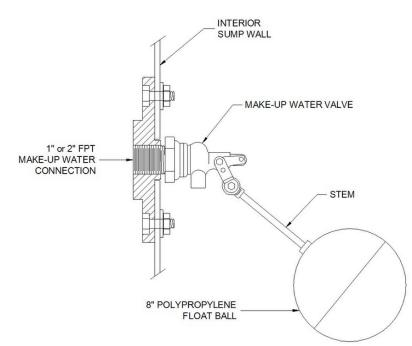
Figure 7 – Mechanical Float Valve
