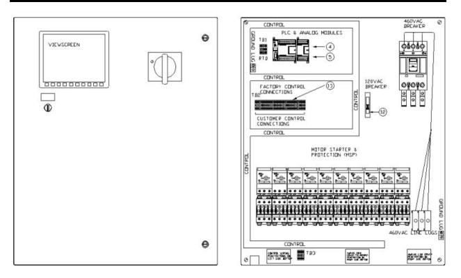
Figure 14 – Typical Motor Control Panel for 10-Fan Cooling Tower Module. (Siemens TOUCH screen standard on all Tower Tech T9900 control panels ordered after August 31, 2011.)
