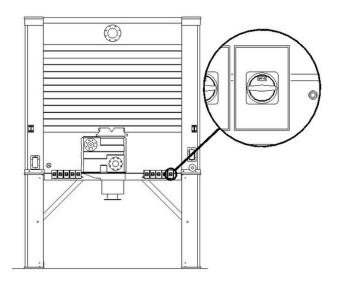
Figure 12 – Optional Rotary-Type Lockout Disconnect Switches
