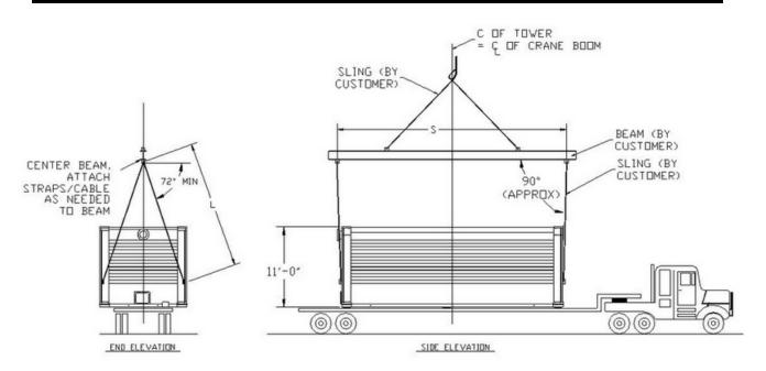
Figure 21 – Tower Lifting Procedure
