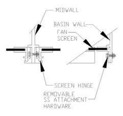
Figure 37 – Close-Up: Fan Guard Hardware
