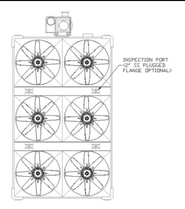
Figure 32 – Mid-Basin Inspection Ports (6-fan tower module shown)
