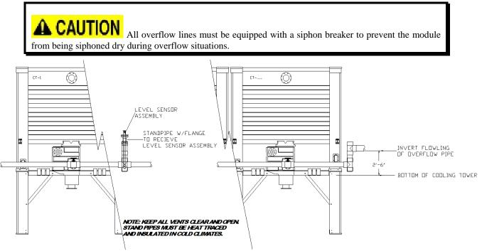
Figure 26 – Typical Overflow/Equalization Piping
