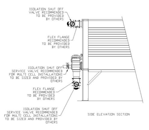
Figure 24 – Connection Flexible Flanges & Flow Control Valves
