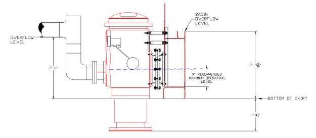
Figure 16B – Sump Level Control Detail
