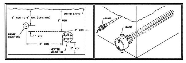
Figure 34 – Location of Basin Heater Probe & Element
