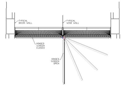
Figure 38 – Opening Fan Guard
