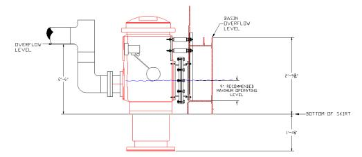
Figure 30 – Sump Level Control Detail
