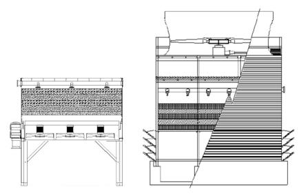
Figure 3 – TTXL versus Conventional Induced-Draft Counter-Flow Tower
