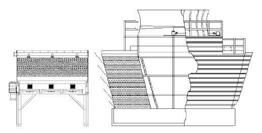
Figure 2 – TTXL versus Conventional Induced-Draft Cross-Flow Tower
