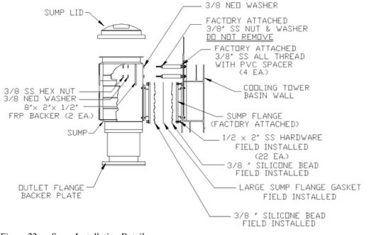
Figure 22 – Sump Installation Detail
