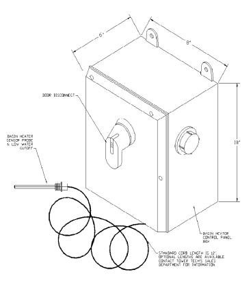
Figure 33 – Basin Heater Control Panel
