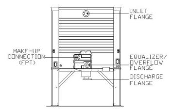
Figure 23 – Standard Piping Connections
