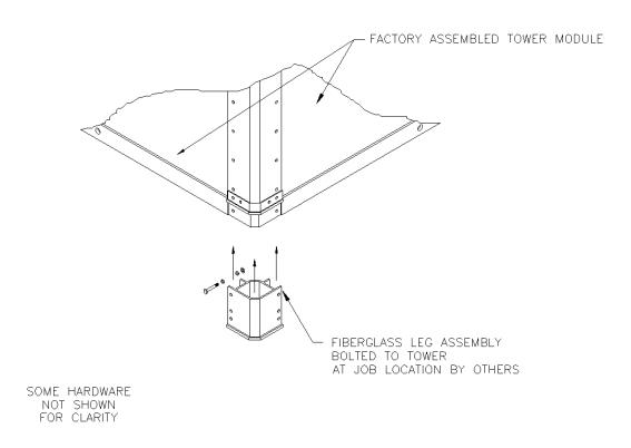
Figure 19 – Installation Detail for 1' Sub-Structure
