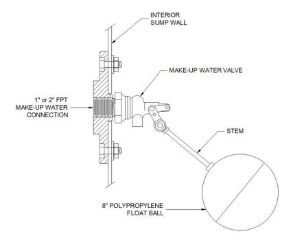
Figure 39 – Mechanical Float Valve
