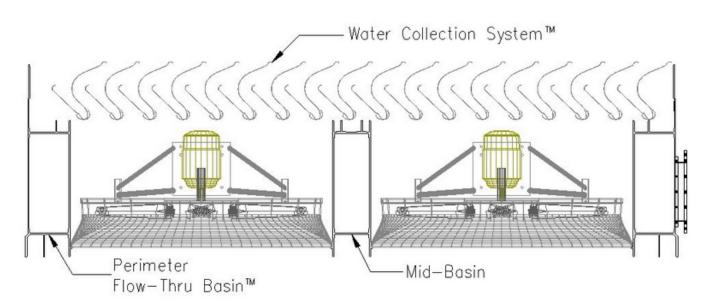
Figure 5 – Water Collection System, Flow-Thru Basin, Mid Basin, Motors, Fans
