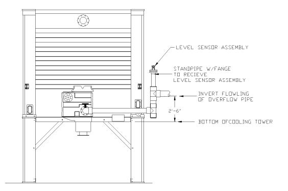
Figure 16A – Ultrasonic Liquid Level Sensor Location
