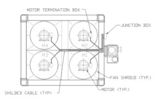
Figure 11 – Typical Wiring Layout
