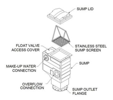
Figure 40 – Sump Layout, Sump Screen Detail
