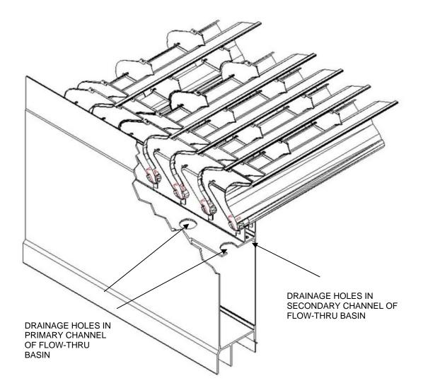
Figure 43 – Flow-Thru Basin Drainage (Perimeter Basin Wall)
