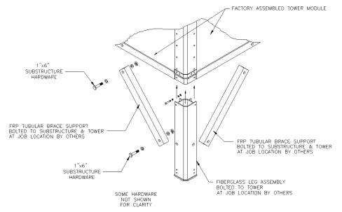
Figure 13 – Tower Sub-Structure
