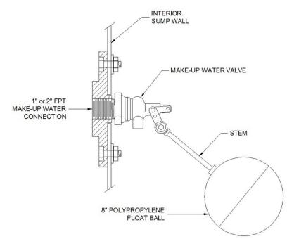
Figure 29 – Mechanical Float Valve
