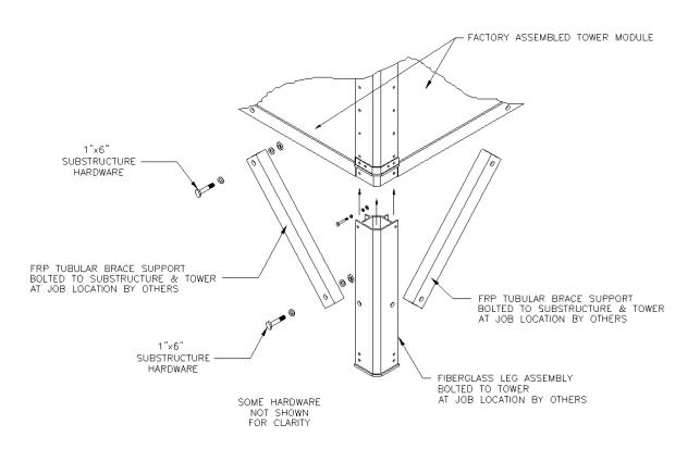
Figure 18 – Installation Detail for Sub-Structures Taller Than One Foot (30.5 cm)
